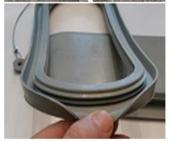
Extended Tongue on cap and grove in flange prevents cap loss during shrinkage due to heat or cold  Deeper locking undercut rings for attachment to corrugated and smooth metal jacketing
